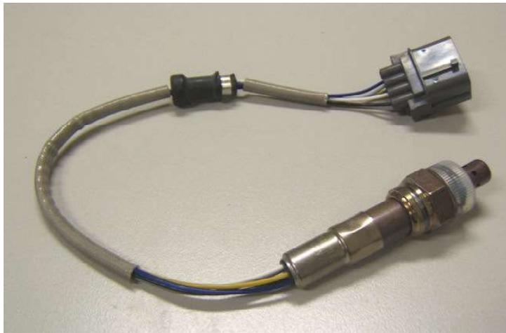
**Note:** the sensor contains a ceramic module and should not be subject to mechanical or thermal shock or it may be damaged.
